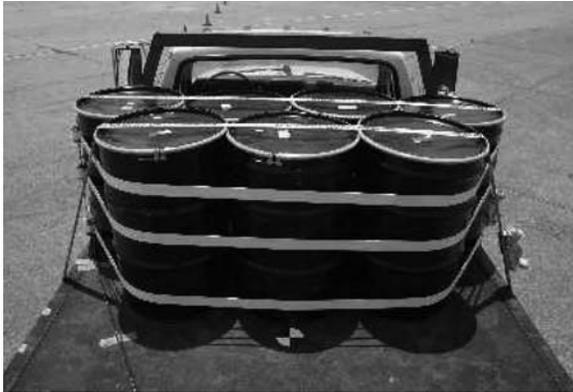
FIG. 2 Typical Ballast Attachment, Rear View
