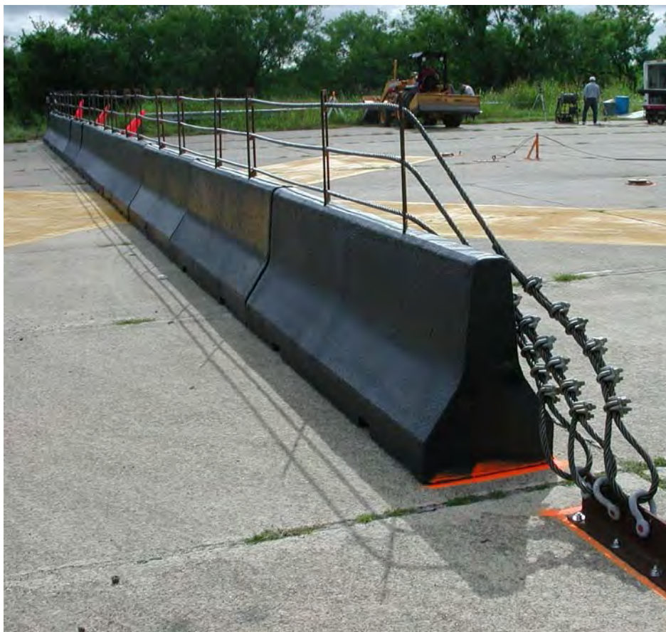
Figure F-4 Polymer-Coated, Lightweight Concrete Barrier System
